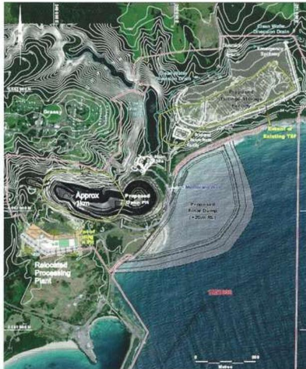
8 year approved open cut mine, average annual production of 400,000 tonnes of ore per annum, yielding 200,000 mtu of WO<sub>3</sub> (1mtu = 10kg)
